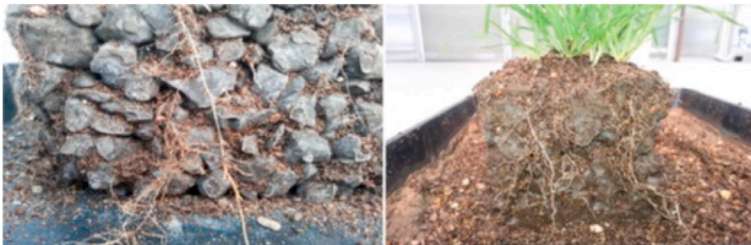
Fig. 9. Root development in porous vegetation concrete [8].
