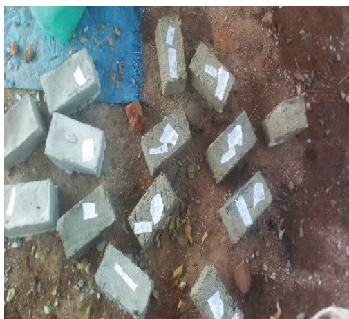
FIGURE 1. Papercrete bricks that were made.
